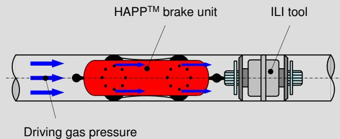
Its hydro-mechanics instantly adapt to any pressure change of the driving gas. Correctly adjusted the brake constitutes a defined counter force to the driving gas force abating all speed variations both above and below the design travel speed.
