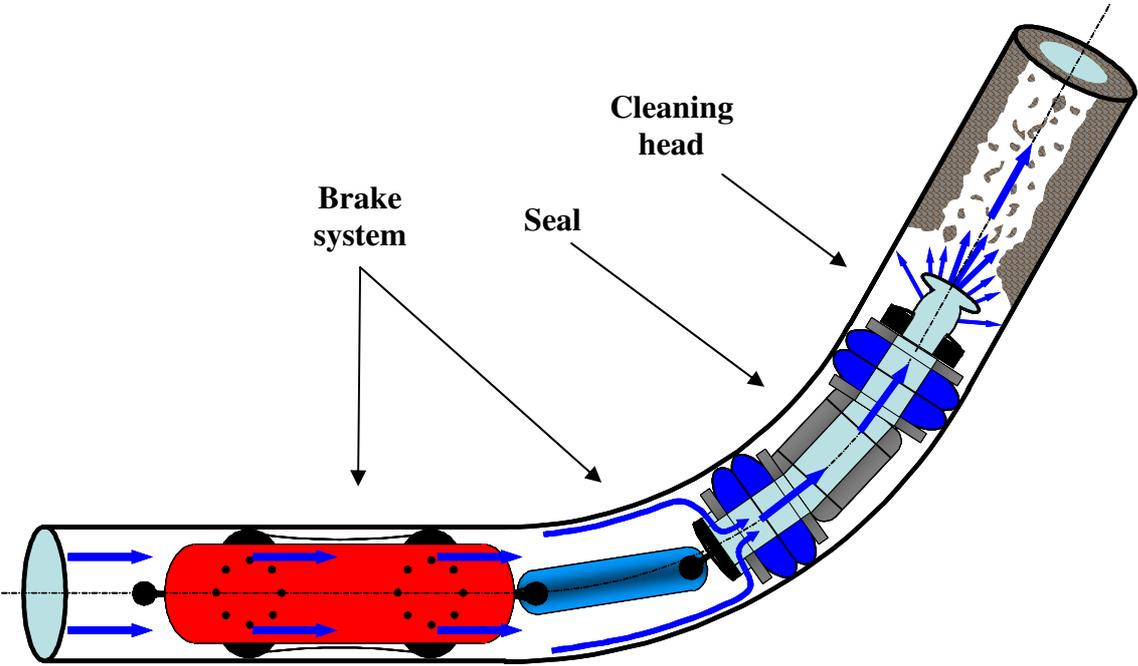
All units have openings that allow the entire fluid flow through the pipeline to bypass. The brake unit ensures that the HAPP is held back against the fluid flow in the pipeline. The fluid pushes against the following seal unit, which channels it into the openings of the cleaning head. Seal unit and cleaning head pose a flow restriction resulting in a pressure difference across HAPP. The fluid is accelerated in the cleaning head's nozzles creating extremely
